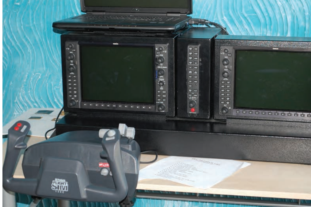
The Garmin G 1000 trainer I used. GATTS configured it to resemble the Aspen EFD 1000 PFD I have in my panel which made the time on the simulator feel comfortable and required minimal transition time.
